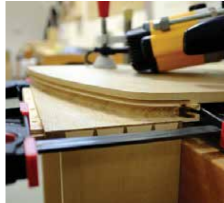
A sacrificial piece of wood is clamped to the side to avoid breakout
