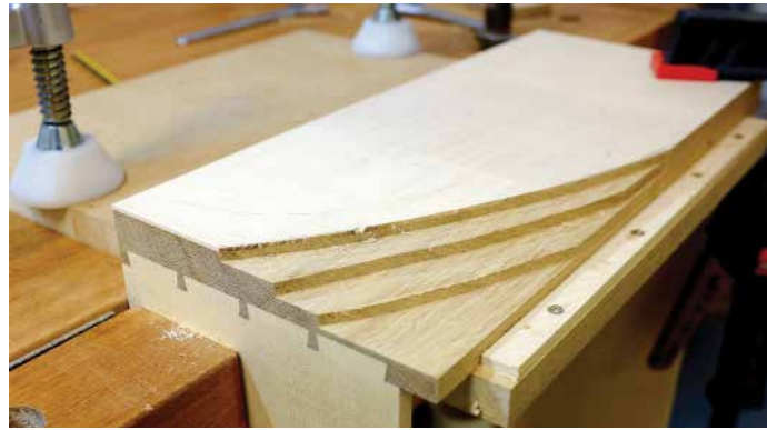
Gradually routing away the front leaving about 5mm from the line
