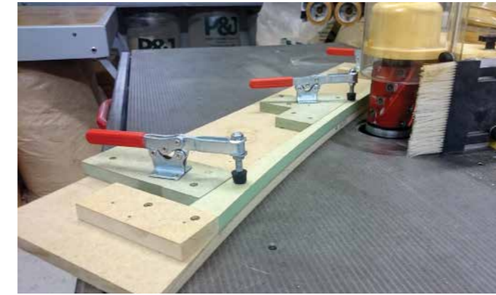
Each MDF strip is spindled to the exact same size
