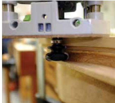
A bearing is added to the bit to run against the template
