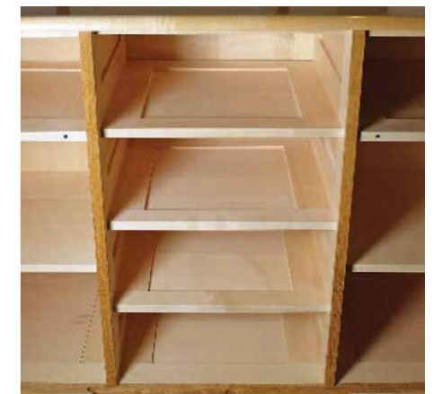
Frame and panel construction
