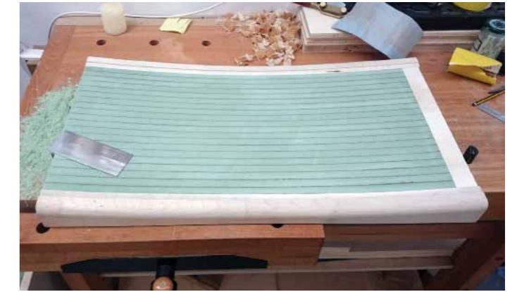
Any discrepancies were taken away by using a stiff card scraper. Wear a dust mask!
