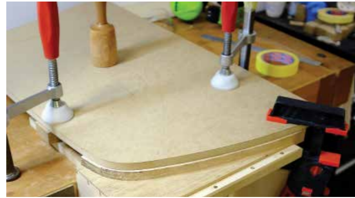
With the template I can rout to the final shape. A Perspex base is added for extra support on the router
